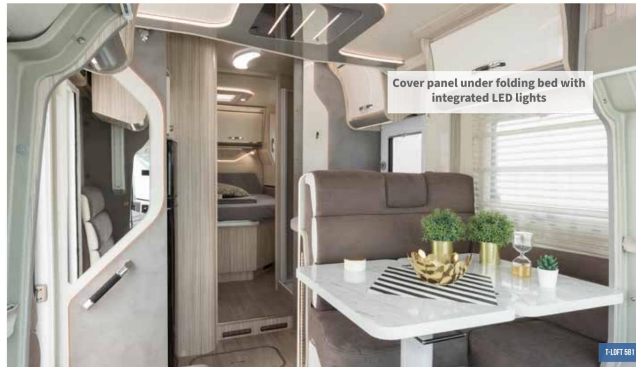
Cover panel under folding bed with integrated LED lights
