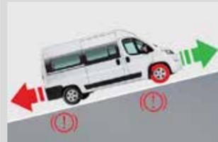
**MSR:** (Motor Schleppmoment Regelung) prevents loss of grip in rough manoeuvres, HBA (Hydraulic Brake Assistance) helps the emergency braking, Hill Holder that keeps the vehicle stationary in the departures uphill.
