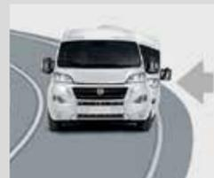
**ESC:** Electronic Stability Control, monitors acceleration, speed and grip. Includes roll-over mitigation, which improves stability by reducing roll, LAC (Load Adaptive Control) supervises the load distribution, ARS which prevents the drive wheels from slipping during acceleration.
