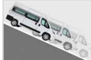
**TRACTION +:** is the device to control the stability of the vehicle in conditions of poor grip of a single driving wheel. Includes Hill Descent Control for controlled speed on steep descents while saving brakes.
